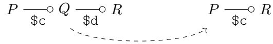
Figure 2.6: Process Q executes the forward \$c = \$d when messages are flowing to the right.
