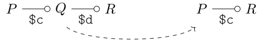
Figure 2.6: Process Q executes the forward \$c = \$d when messages are flowing to the right.
